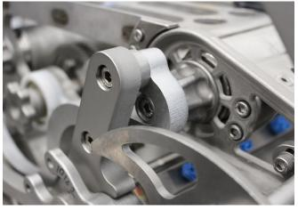
Elliði Hreinsson shows off the newest Curio C-2034 filleting machine featuring over 100 metal parts 3D printed on the Desktop Metal Studio System.
