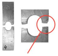
Failure: always about the hole Traditional method to increase
