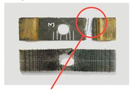
Failure: in the regular zone — part is equally strengthened
